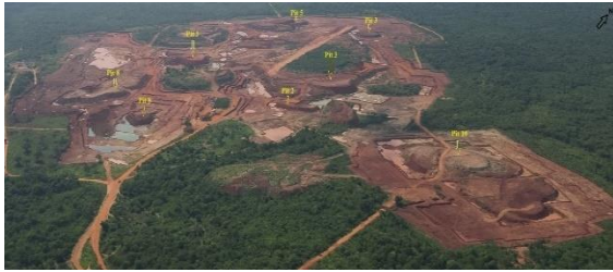
Figure M15: In-pit backfilling at Mugloto Pits
